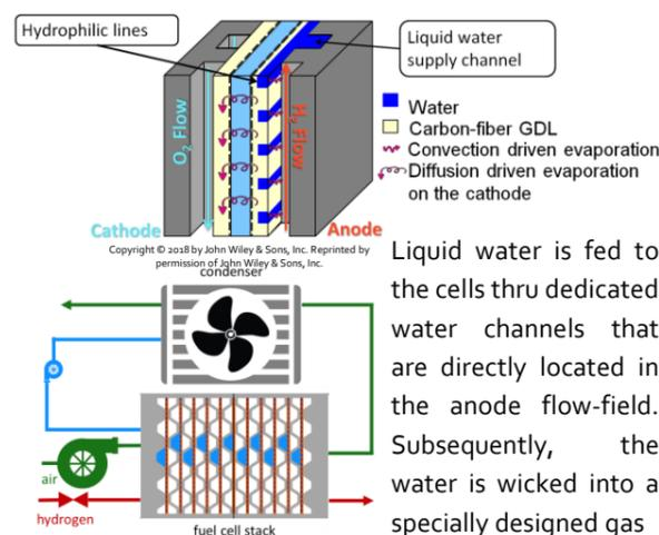
Liquid water is fed to the cells thru dedicated water channels that are directly located in the anode flow-field. Subsequently, the water is wicked into a specially designed gas diffusion layer (GDL) with a mixed hydrophilic and hydrophobic pattern [4,5] and distributed through the entire cross-section. Consequently, the water evaporates, cools the cell by taking up the heat of evaporation and is released as water vapor.
