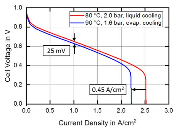
Simulation results show that operating conditions which are favorable for evaporative cooling (i.e. 90 °C, 1.6 bar) show a slightly decreased electrochemical performance compared to conventional operating conditions (80 °C and 2 bar)
