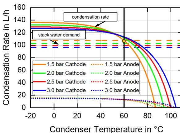
Ideal condensation rate increases with decreasing condenser outlet temperature. Intersection with stack water demand yields necessary condenser outlet temperature (e.g. 60 °C in above example).
