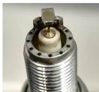
Figure 1: M10 optical spark plug with two fibers dedicated to spark-induced breakdown spectroscopy
