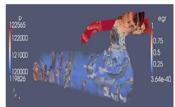
Fig. 4 CFD simulations results – pressure and EGR
