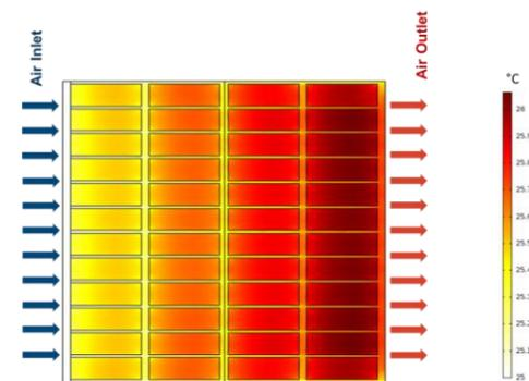
Most important to reach also homogeneous temperatures between different Li-ion cells inside a battery pack, the cooling air flow velocity has to be equal between different flow channels. If this is realized, the heat transfer from the cell surfaces to the air flow will be the same.
