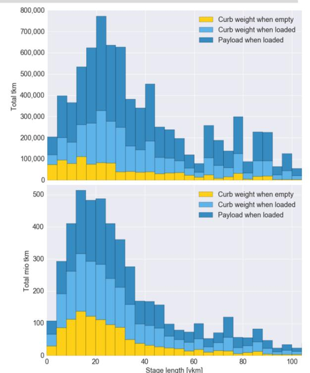
Figure 2: Sum of tkm performance by stage (constant payload) length. Blue bars are tkm in loaded stages, yellow bars are tkm in empty ones. Also the curb weight of the truck accounts to the tkm. Top: single construction company. Bottom: all truck from GTE in 'stone and earth' business. From the higher share of dark blue bars it is possible to infer that the construction company is optimizing its logistics better than its competitors.
