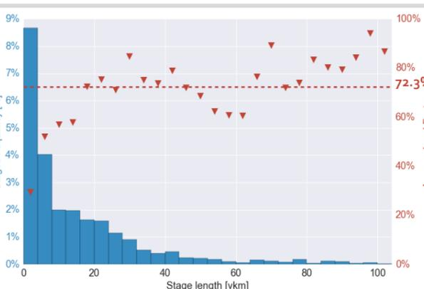
Figure 4: Blue bars: relative frequency of stages by stage length. Red triangles: average loading factor for those stages. Dashed line: overall average loading factor.
