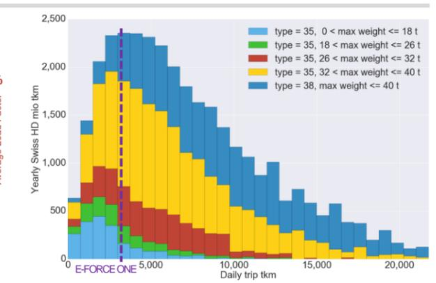
Figure 5: X-axis: effective tkm (curb weight + payload) performed by a truck in a day (= trip). Y-axis: sum of tkm of all trips within a range of daily tkm performance, by truck type and maximum permissible weight.
