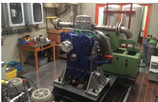
Fig.4: View of the 1-cylinder research engine test-rig
